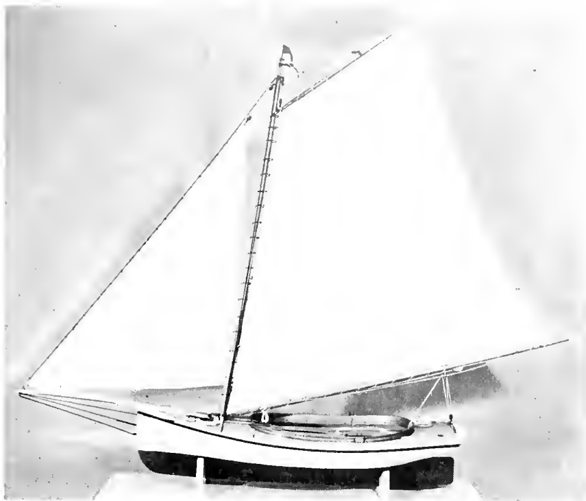
CENTERBOARD NOANK SLOOP of the type used in the lobster fishery on Long Island Sound, 1875-1900. Rigged model USNM 26804. (Smithsonian photo 47607 d.)
